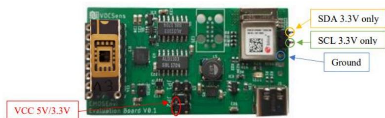
Figure 6. EvaBoard connection for I2C use.
